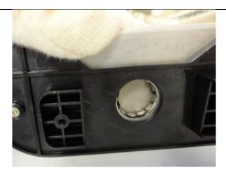
Step 8: Install the lock mechanism on the other side using the two phillips screws.
