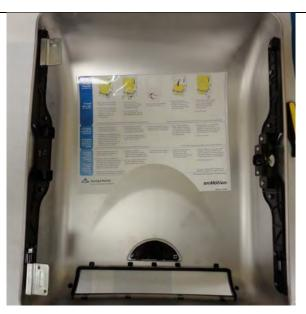
**Step 9:** Install the cover back onto the dispenser using the four torx screws in the locations circled in orange.
