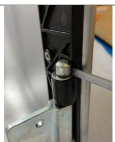
**Step 4:** Install the hinges on the opposite side and pop the snap rings in place.
