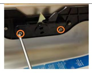
**Step 6:** Remove the hole plug by pressing against it with the large flat head screwdriver.
