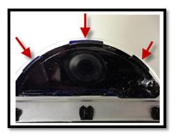
2. Snap the lens in place by gently applying pressure near the bottom of the lens from the outside of the cover. (Picture #2). To ensure the lens is securely installed, gently press around the entire perimeter of the lens.
